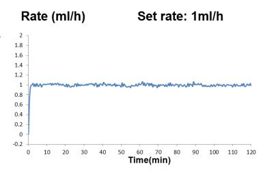
Syringe brand: Dove Syringe specification: 20ml Sampling quantity of pump: 3 Sampling quantity of syringe: 3
